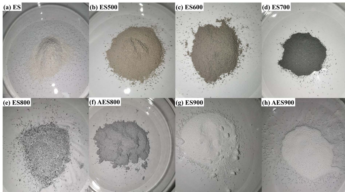
Fig. 1 The digital photo of raw eggshells (a), eggshells after heating at 500 (b), 600 (c), 700 (d), 800 (e) and 900 °C (g), and heated eggshells after aging (f) and (h).
