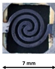
Figure 6. A picture of the PreHG after the deposition of the adsorbent material on its surface.
