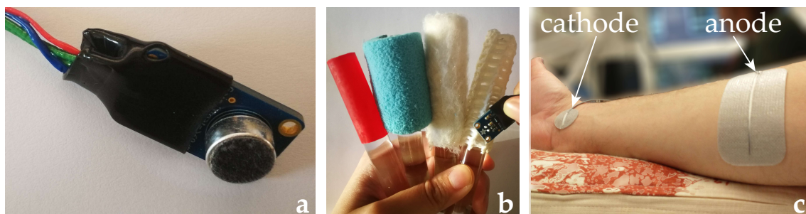
Figure 1. (a) Close-up image of the omnidirectional electret condenser microphone with an amplifier module. An isolation cable was put on the circuit board for an easier grip of the microphone during the stroking and to reduce interference with the components on the printed circuit board (PCB). (b) The experimenter was stroking the different textures with a microphone in a proximal to distal direction. (c) Placement of the electrodes on the participant's forearm. The cathode was placed over the median nerve while the anode was applied on the upper part of the forearm.
