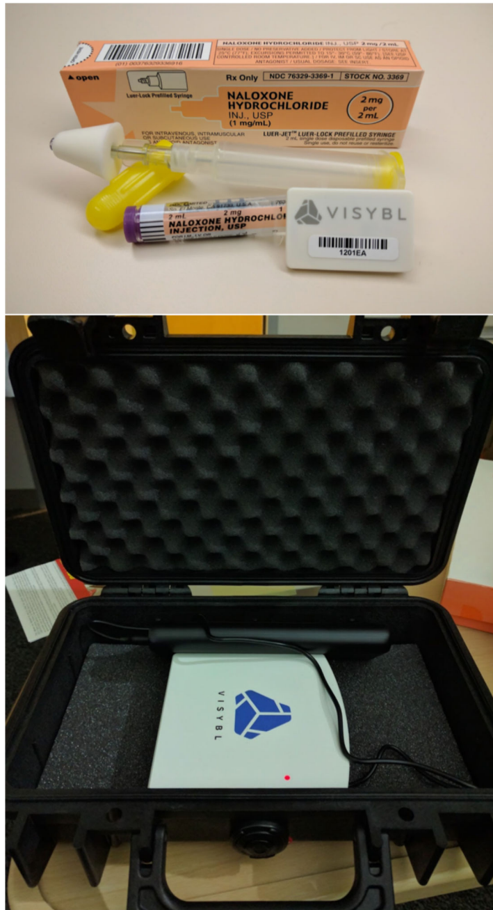
Figure 2. Smart naloxone kit consisting of naloxone ampoule, syringe, nasal mucosal atomizer device, and BLE beacon (top). BLE reader, portable battery pack, and shockproof casing (bottom).
