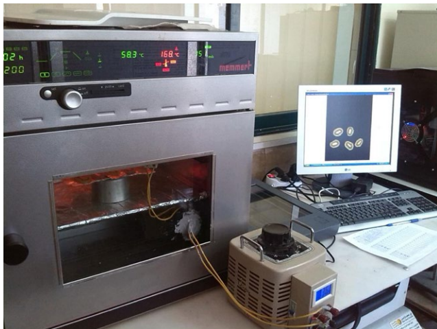
FIGURE 1 A schematic of the infrared-vacuum dryer
