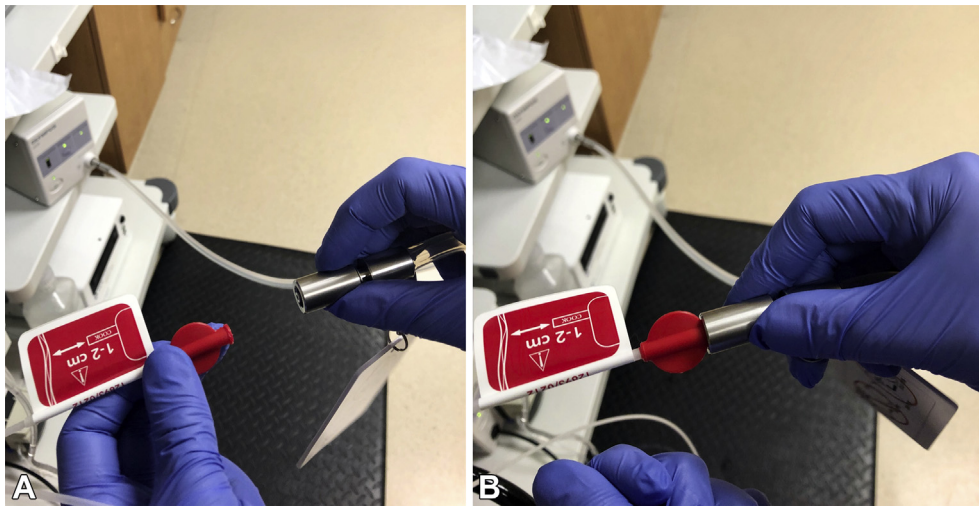
Figure 2. The A , red end of the TC-325 (Hemospray) delivery catheter is then B , connected the the free end of the CO 2 tubing.
