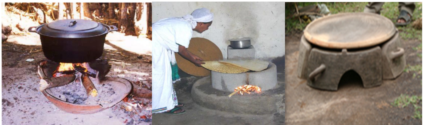
Figure 3. Cooking stove (a) three stone open fire and injera baking stove (b) mirt (c) gonze in Ethiopia.
