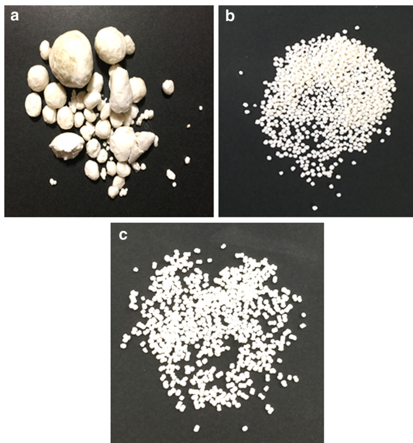
Fig. 3. Image (a) of agglomerated product after spheronizing a formulation (naproxen, Tween 80, Avicel, and Aerosil) containing high water content and longer threads. Image (b) of good quality pellets (spherical particles with less size variation) after spheronizing a formulation (naproxen, PG, Avicel, and Aerosil) containing lower water content and shorter threads. Image (c) of reasonable quality pellets (dumbbell shape would be considered less quality but reasonable) of physical mixture formulation (naproxen, Avicel, and Aerosil)
