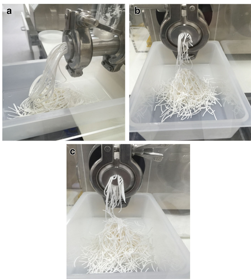
Fig. 2. Image (a) of extrudate of a formulation (naproxen, Tween 80, Avicel, and Aerosil) containing high water content, exhibiting high plasticity. Image (b) of extrudate of a formulation (naproxen, PG, Avicel, and Aerosil) containing lower water content, exhibiting lower plasticity. Image (c) of extrudate of physical mixture formulation (naproxen, Avicel, and Aerosil)
