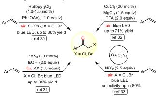
20 mol % catalyst loading and the combination of MgCl $_2$  (1.5 equiv) and TFA (2 equiv). A copper-modified graphite carbon nitride (Cu–C $_3$ N $_4$ ) mediated heterogeneous photocatalysis was also reported for the oxohalogenation of styrenes under visible-light irradiation, employing stoichiometric amounts of NiX $_2$  (X = Cl, Br) as the halide source. 3
