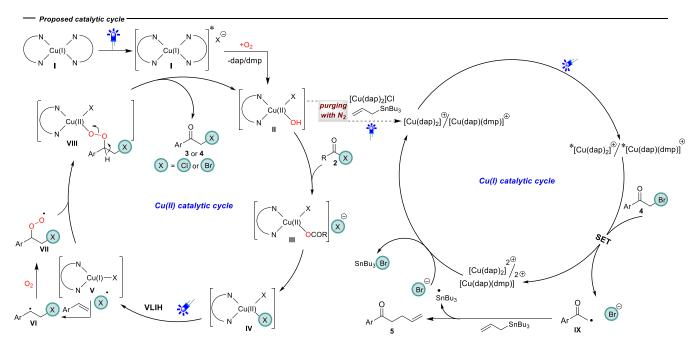
or 4 with concurrent elimination of II from VIII closes the catalytic cycle. In turn, Cu(I) activates the haloketone 4 via SET to form radical IX, which engages in an ATRA process following established lines.<sup>21</sup> However, involvement of a heteroleptic Cu(I)(dap)(dmp) complex is also possible for the Cu(I) photocatalyzed oxoallylation step as revealed by the <sup>1</sup>H NMR experiment (see the SI).
