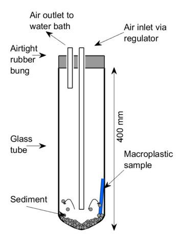
Supplementary Figure S1: Schematic diagram of abrasion chamber apparatus used for the experiments. Air velocity at the base of the inlet is 11.7 m s-1. Sediment particle velocity within the chamber is c. 0.63 m s<sup>-1</sup>
