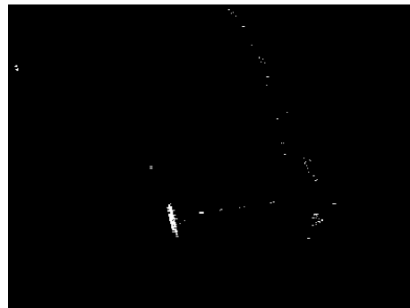
Figure 7. Detection result of the cell-averaging constant false alarm rate (CA-CFAR) detector for the chosen SSDD image.
