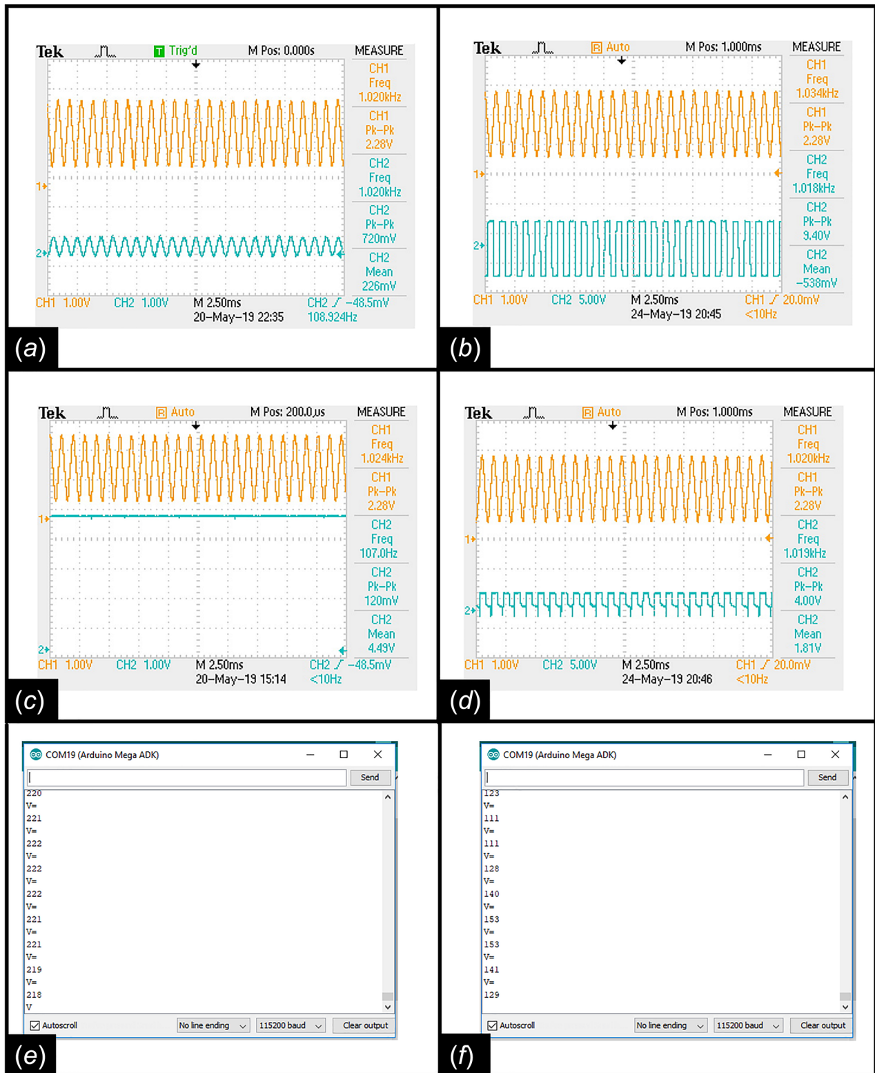
Fig. 8 Testing of the loose-lead monitoring system. (a) Differential voltage signal across active electrode-formulation-diffusion media-electrode arrangement when the electrodes were properly connected, (b) differential voltage signal across active electrode-formulation-diffusion media-electrode arrangement when one of the electrodes was displaced, (c) output of the comparator circuit when the electrodes were properly connected, (d) output of the comparator circuit when one of the electrodes was displaced, (e) the serial monitor reading when the electrodes were properly connected, and (f) the serial monitor reading when one of the electrodes was displaced (note: the upper waveform represents the output from the signal generator; the lower waveform represents the output at various stages of the circuit).
