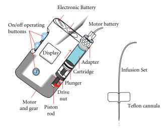
FIGURE 3: Main parts of an insulin pump.
