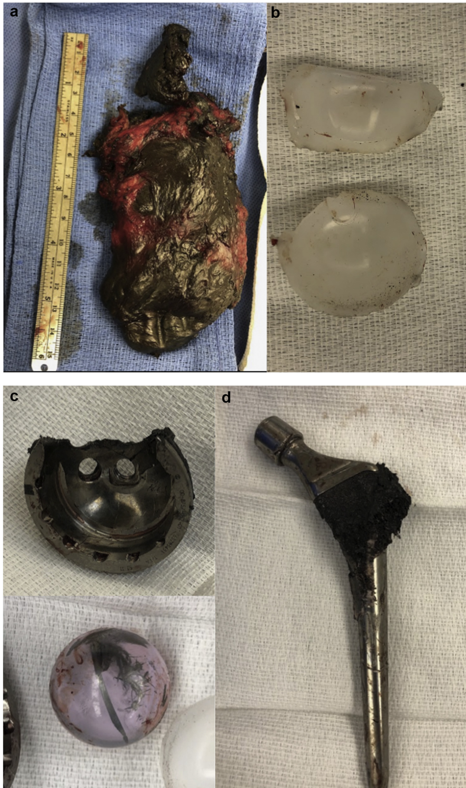
Figure 3. Clinical photographs of the resected hip pseudotumor (a), fractured polyethylene liner (b), femoral head and acetabular shell with extensive erosion at the point of contact (c), and femoral stem with retained trunnion and extensive metallosis (d).
