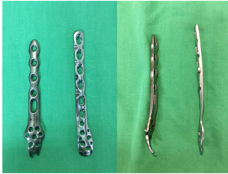
Fig. 1 The two low-profile and anatomical periarticular locking plates used in this study
