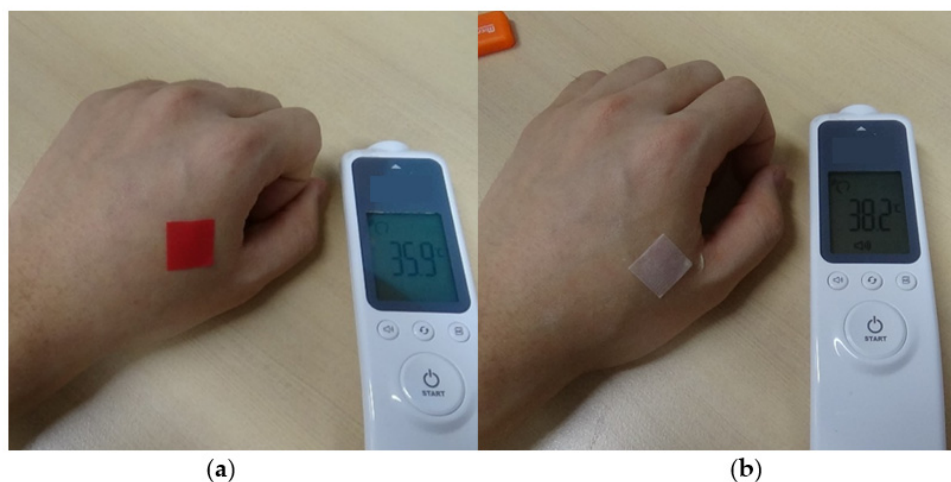
Figure 15. Patch attached to the skin on the back of the hand with different temperatures: (a) normal temperature condition and (b) fever condition.
