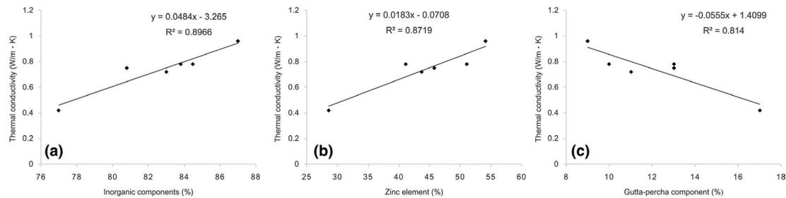
**FIGURE 2** The simple linear regression analyses. (a) The correlation between thermal conductivity and inorganic components. (b) The correlation between thermal conductivity and zinc element. (c) The correlation between thermal conductivity and gutta-percha component.
