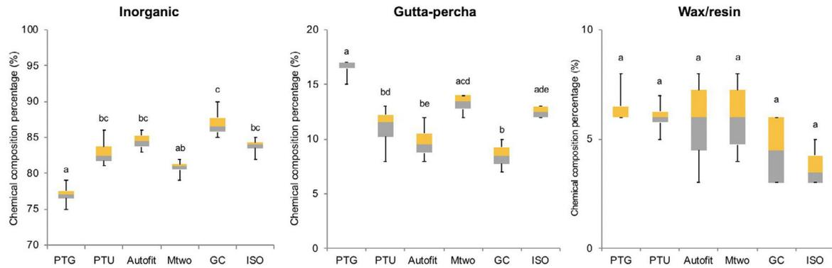
**FIGURE 1** Box plot of inorganic, gutta-percha and wax/resin components of commercial dental gutta-percha points. Different lowercase superscript letters indicate significant differences according to the Kruskal–Wallis and Dunn tests ( $p < .05$ ). [Colour figure can be viewed at wileyonlinelibrary.com]
