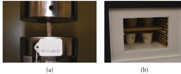
FIGURE 2: (a) Compression testing. (b) Bone ashing.
