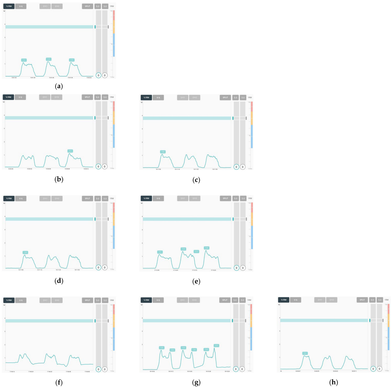
Figure 9. Images of collected sEMG signals by different types of embroidery-based textile electrodes with wearable devices. (a) Reference; (b) CS_1; (c) CS_2; (d) Em_LS; (e) EM_Ms; (f) Kn_PL; (g) Kn_PU; (h) Kn_IN.
