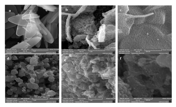
**Figure 1.** SEM images of ZIF-67 prepared in different solvents: (**a**) ZIF-67 prepared in H<sub>2</sub>O, before pyrolysis, after pyrolysis; (**b**) NPC/CO (H<sub>2</sub>O) at 700 °C; (**c**) NPC/CS (H<sub>2</sub>O); (**d**) ZIF-67 prepared in MeOH; (**e**) NPC/CO (MeOH) at 700 °C; and (**f**) NPC/CS (MeOH).
