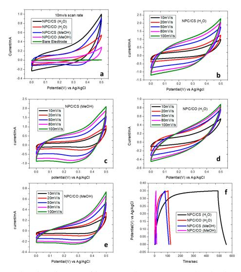
**Figure 6.** Electrochemical properties of the NPC/CO and NPC/CS in 2M KOH: (**a**) cyclic voltammetry at 10 mv/s scan rate (**b**–**e**) at different scan rates and (**f**) charge-discharge profiles at 0.01 mA/g.
