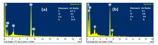
Figure 3. EDS spectrum of (a) NPC/CS (H2O) and (b) NPC/CS (MeOH).
