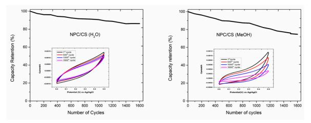
**Figure 7.** Numbers of cycles versus capacitive retention for the electrode NPC/CS electrode materials recorded over 1600 cycles at a scan rate of 100 mV/s.
