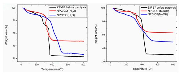
Figure 4. TGA curve analysis of as prepared ZIF-67, NPC/CO, and NPC/CS.
