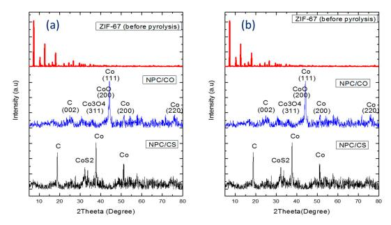
**Figure 2.** XRD patterns of (**a**) ZIF-67, NPC/CO and NPC/CS prepared in H2O and (**b**) ZIF-67, NPC/CO, and NPC/CS prepared in MeOH.
