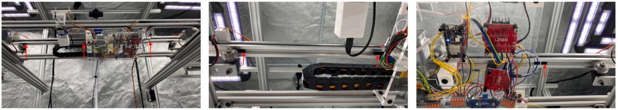
Fig. 19. Image showing V-slot covers in the mover arm that is used to localise the arm positions. This is annotated in red. An overview is shown on the left and the zoomed in view is shown in the middle and on the right. There are three V-slot cover markers in total. (For interpretation of the references to colour in this figure legend, the reader is referred to the web version of this article.)
