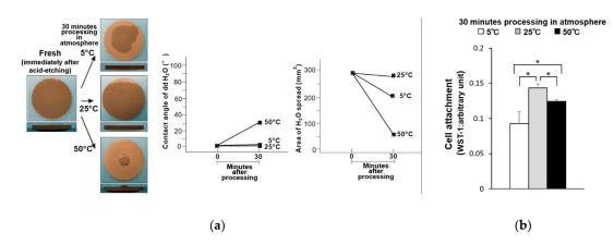
**Figure 3.** (a) Hydrophobicity/hydrophilicity of the fresh–dry titanium disk surfaces illustrated as a photograph of  $10 \,\mu$ L ddH<sub>2</sub>O placed on the sample surface before and after temperature deviation (left) with the corresponding contact angle (middle) and spread area (right). (b) Initial attachment of osteoblasts to the fresh–dry titanium disk surfaces. \* *p* < 0.05, statistically significant difference.
