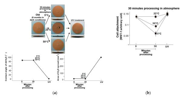
**Figure 7.** (a) Hydrophobicity/hydrophilicity of the UV-treated old–dry titanium disk surfaces illustrated as a photograph of  $10 \ \mu L \ ddH_2O$  placed on the sample surface before and after temperature deviation (upper middle) with the corresponding contact angle (lower left) and spread area (lower right). (b) Initial attachment of osteoblasts to the UV-treated old–dry titanium disk surfaces.
