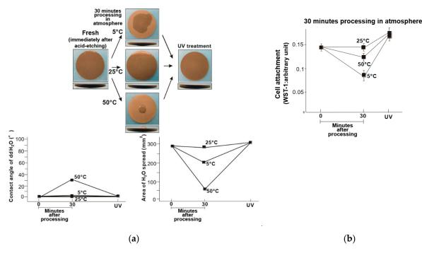
**Figure 8.** (a) Hydrophobicity/hydrophilicity of the UV-treated fresh–dry titanium disk surfaces illustrated as a photograph of 10  $\mu$ L ddH<sub>2</sub>O placed on the sample surface before and after temperature deviation (upper middle) with the corresponding contact angle (lower left) and spread area (lower right). (b) Initial attachment of osteoblasts to the UV-treated fresh–dry titanium disk surfaces.
