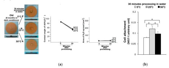
**Figure 2.** (a) Hydrophobicity/hydrophilicity of the old–wet titanium disk surfaces illustrated as a photograph of  $10 \,\mu\text{L}$  ddH<sub>2</sub>O placed on the sample surface before and after temperature deviation (left) with the corresponding contact angle (middle) and spread area (right). (b) Initial attachment of osteoblasts to the old–wet titanium disk surfaces. \* p < 0.05, statistically significant difference.
