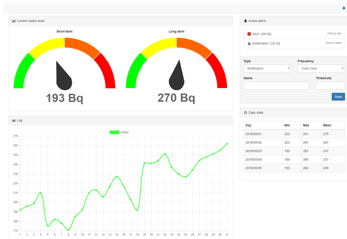
Figure 7. Dashboard of the radon gas monitoring system.
