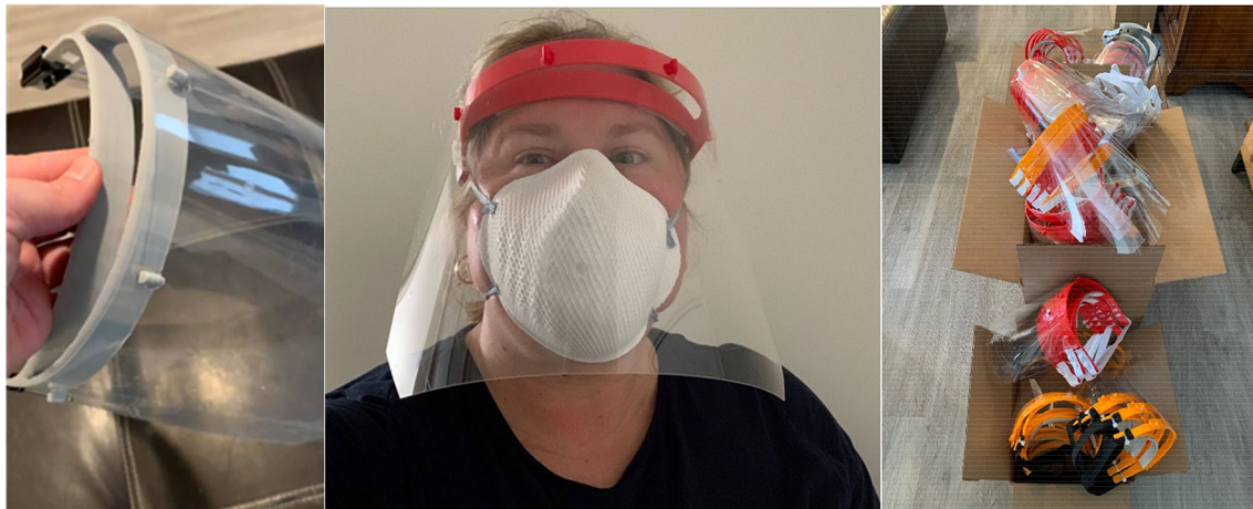
FIGURE 3. Drexel AJFlex Face shield with parts / components: headband, shield material, elastic banding around the back of the head, zip ties to secure the elastic material to the headband, and thin foam strip on the inner surface of the headband for comfort along the forehead.
