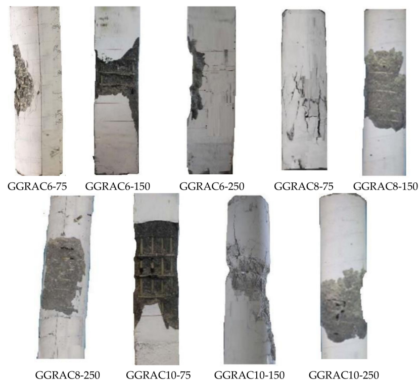
Figure 5. Crack initiation of GGRAC compressive members.
