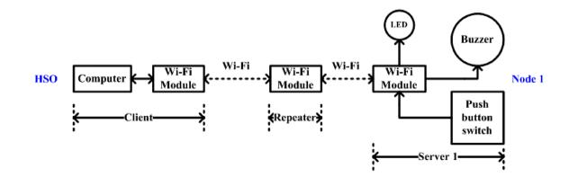
Fig. 3 Detailed block diagram of the communication between one individual server with client
