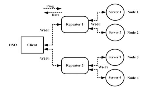
In this study, the authors consider the client has two repeaters (repeater 1 and 2). Repeater 1 has two servers (server 1 and 2), and repeater 2 has two servers (server 3 and 4). The client randomly pings to the respective repeaters. These
