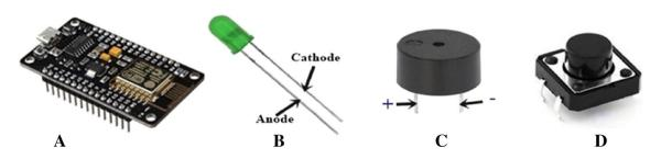
Fig. 5 Components used for prototype development. a NodeMCU (ESP8266), b LED, c Buzzer, and d Push button switch
