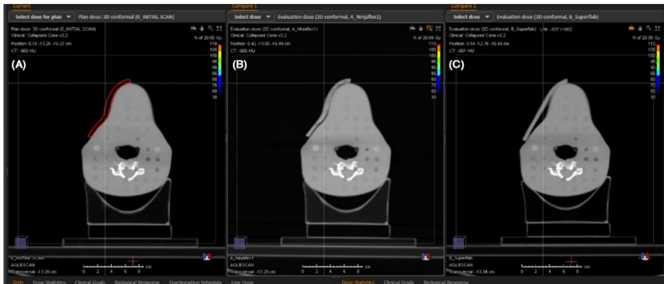
FIG. 3. Conformity to skin surface from left to right Bolus Virt , Ninjaflex1 and Superflab.
