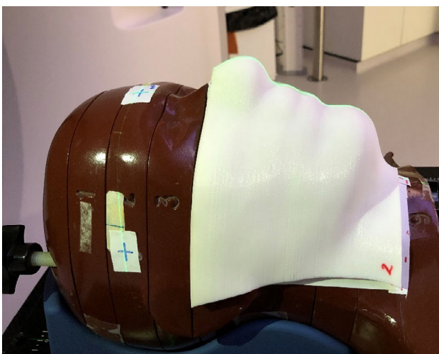
Fig. 1. Positioning of three-dimensional printed Ninjaflex bolus covering the right-hand side of the head phantom to include the nose, lips, chin, and mandible.
