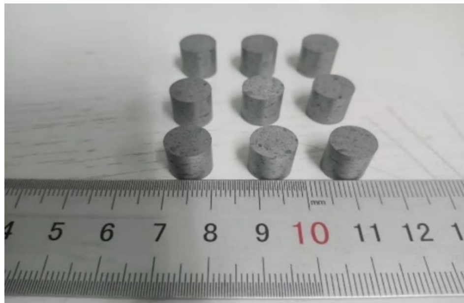
Figure 2. Physical drawings of some Al-rich Al/PTFE/TiH 2 experimental specimens.
