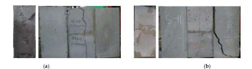
Figure 7. Shear failure pattern of AAC block masonry: (a) S1-3; (b) S2-5.
