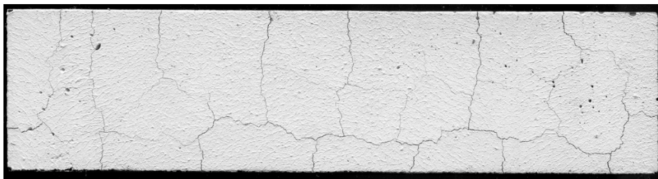
Figure 3. Cracking pattern on the surface of the cement matrix with MWCNTs (C52CNT) with w/c = 0.4.
