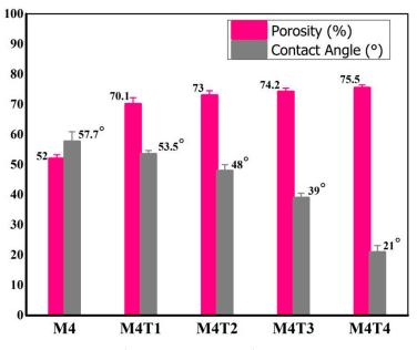
**Figure 5.** Pristine and nanocomposite membranes' static water contact angle (average contact angles of samples are reported) and percent porosity.
