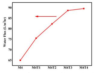
Figure 8. Water flux measurements of the prepared membrane with or without  $TiO_2$ /pore former.
