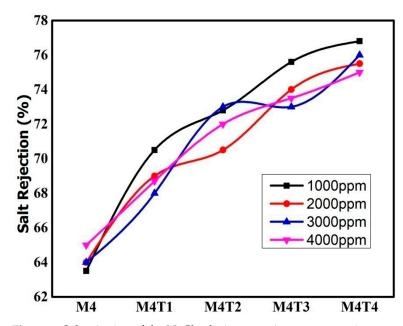
Figure 9. Salt rejection of the NaCl solution at various concentrations.
