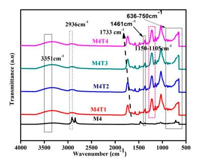
Figure 2. FTIR spectrum of the fabricated nanocomposite membranes.
