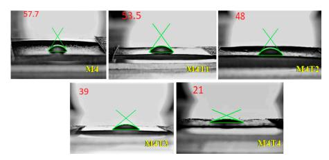
Figure 6. Static water contact angles: M4, M4T1, M4T2, M4T3, and M4T4.
