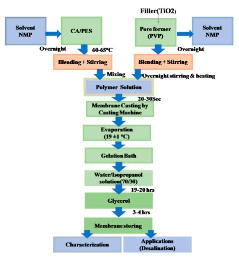
Figure 1. Preparation method of the mixed-matrix nanocomposite membranes.
