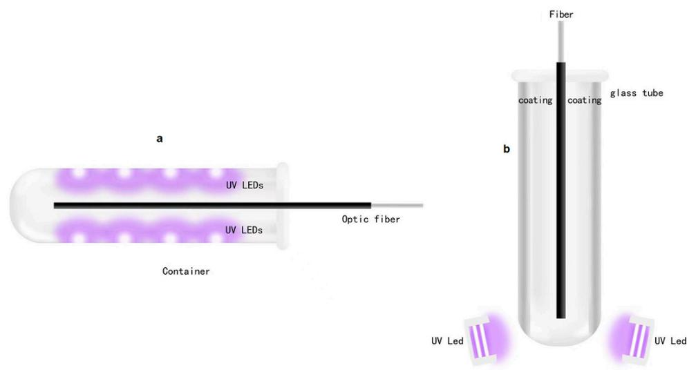
**Figure 4.** Preliminary design (a), sketch of coating (b).
