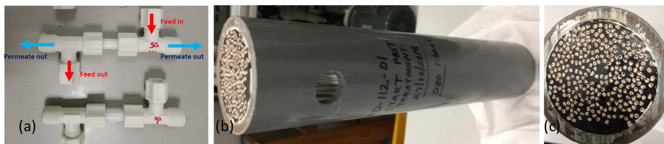
Figure 1. Scale up of tri-bore hollow fiber membrane modules. (a) Lab-scale testing modules (0.5-inch diameter), (b,c) pilot-scale modules (2-inch diameter).
