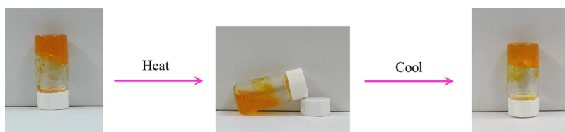
Figure 6. Reversible sol–gel transition of Gel-D induced by temperature stimuli. Photograph courtesy of Nan Hou. Copyright 2020.
