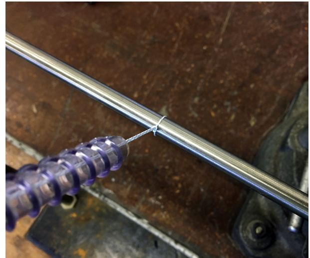
Fig 1. Knot-tying cannula setup. Knots were tied through a standard arthroscopic cannula using a knot pusher, onto the 30-mm dowel.
