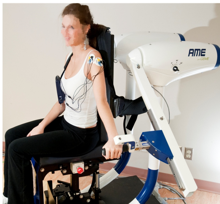
Figure 2. The AME device (Appareil Multifonctionnel d’Entraînement—multifunctional training device): a patient is conducting an abduction exercise with the placement of surface EMG electrodes on the shoulder.
