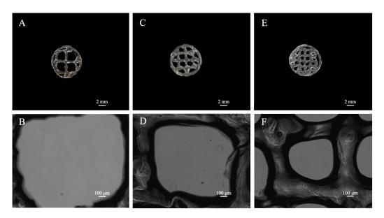
**Figure 4.** 3D bioprinted scaffold template. Camera pictures ((**A**,**C**,**E**)—Scale bar 2 mm—Magnification  $5\times$ ) and light microscope images ((**B**,**D**,**F**)—Scale bar  $100 \mu m$ ), respectively, for the circular shape with 35, 50, and 75% level of grid filling.
