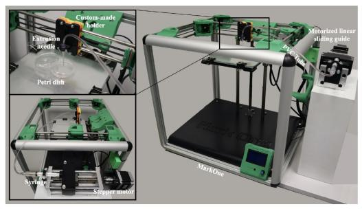
Figure 2. Final layout of the custom-made 3D bioplotter.
