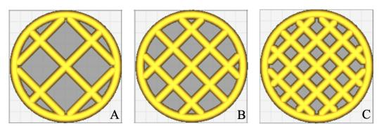
**Figure 1.** Circular shape with 35 (**A**), 50 (**B**), and 75 (**C**) % level of grid filling.
