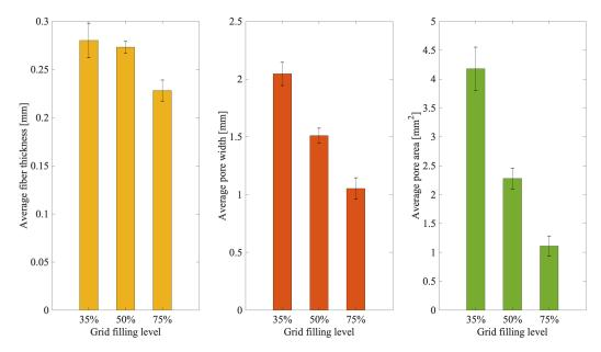
**Figure 5.** Evaluation of the 3D bioprinted scaffold templates with different grid fillings. (**Left panel**), fiber thickness; (**middle panel**), pore width; (**right panel**), pore area.
