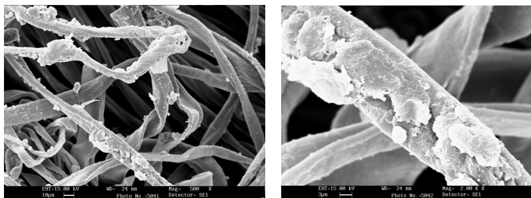
Figure 5. SEM image of fabric impregnated with formulation P25M4.56, at magnification 500× (left) and 2000× (right).
