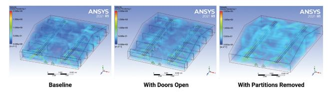
Figure 8. Velocity [m/s] distribution of the three investigated cases (L: doors closed [baseline], M: with the doors open, R: with the partitions fully removed).
