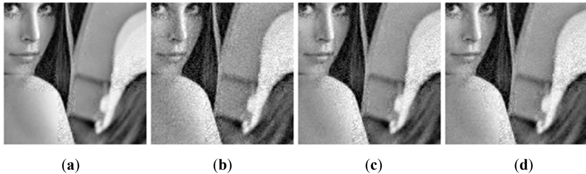
Figure 13. Subjective comparison (PSNR) of portions of Lena ( SR = 0.7 , R = 5 ) after CS reconstruction. (a) no quantization (27.92 dB); (b) uniform quantization (24.34 dB); (c) PDF-based quantization (26.32 dB); (d) universal quantization (26.13 dB).
