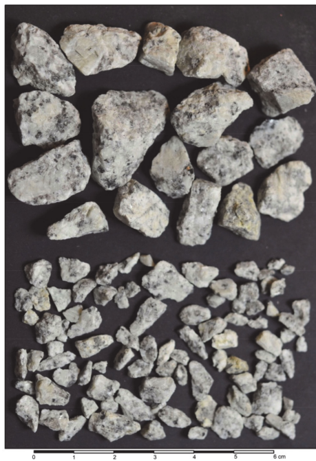
Figure 2. Granite fragments of coarse aggregates: medium and fine gravel.
