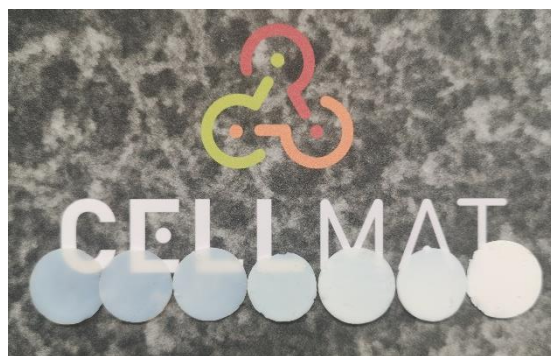
Figure 6. Photograph of the aerogels under study. From left to right: 1, 3, 4, 6, 8, 15 and 20 wt.% of catalyst content.
