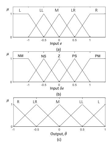
**Figure 10.** Input and output membership functions of fuzzy inference system. (**a**,**b**) The input membership functions. (**c**) The output membership function. The fuzzy labels are defined as R: Right, LR: Little Right, M: Middle, LL: Little Left, L: Left, NM: Negative Medium, NS: Negative Small, Z: Zero, PS: Positive Small, and PM: Positive Medium. It should be noted that the membership functions are given in normalized scales.
