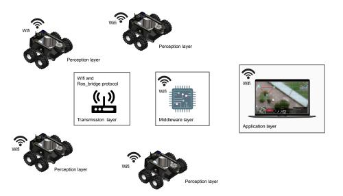
Figure 7. Overview for a Raptor drain inspection system.
