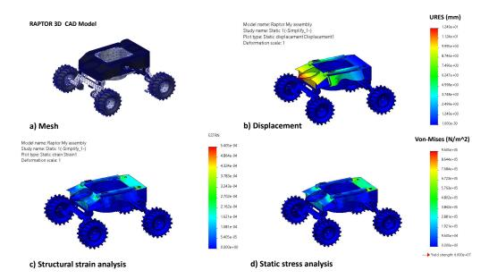
**Figure 5.** Static structural analysis (**a**) Tetrahedral mesh of Raptor 3D model (**b**) Static Displacement analysis (**c**) Strain Analysis results (**d**) Von Mises stress in N/m<sup>2</sup>.
