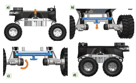
**Figure 2.** Steps of the reconfiguration. (**a**) Push button pressing to open the provision to insert and hold the pin (**b**) Pulling the lock open when triggering the pull lever (**c**) Adjusting the wheel assemblies (**d**) New wheel assembly configuration
