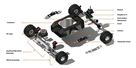
a diameter of 20 mm, the motor is compact and power-packed. All-wheel drive enables faster turning and easier obstacle crossing.
