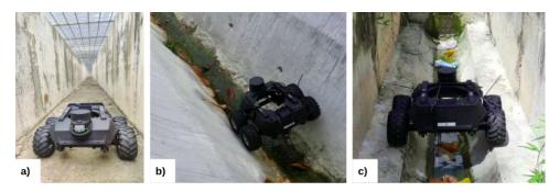
**Figure 3.** Adaptability of the robot to various drain scenarios. (**a**) In a drain with a flat floor (**b**) In a drain with a curved bottom (**c**) In a cut-off drain
