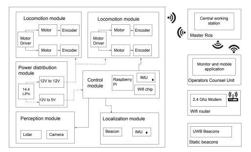
Figure 6. Control Architecture.
