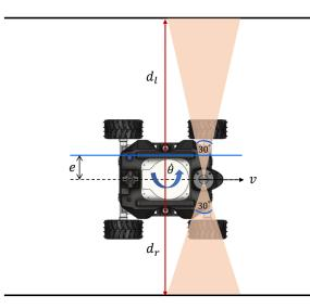
Figure 9. Principle of navigating in the middle of a drain.
