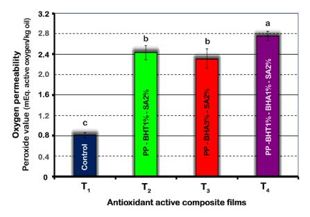
**Figure 3.** Effect of composition of polypropylene-based films on oxygen permeability of composite films. Means (n = 3) with different letters are significantly different (p < 0.05). Error bars corresponding to standard deviations.
