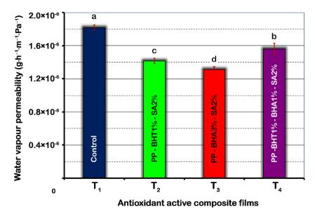
**Figure 1.** Effect of composition of polypropylene-based films on water vapour permeability (WVP). Means (n = 5) with different letters are significantly different (p < 0.05). Error bars corresponding to standard deviations.
