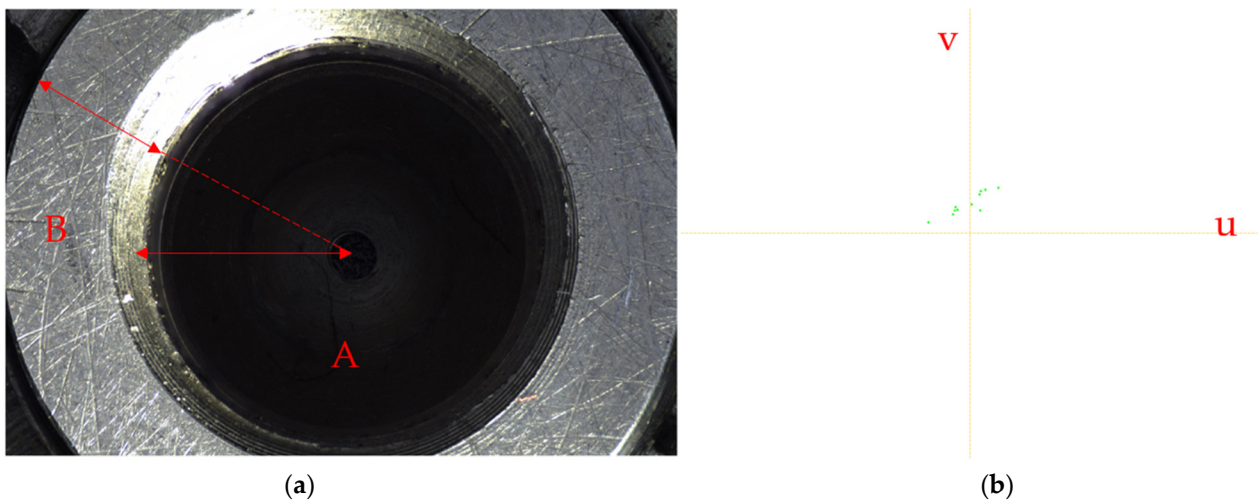
Figure 4. Texture region segmentation of fuel nozzle. (a) Segmentation of fuel nozzle. A refers to the inlet hole. B refers to the area of the entrance annular (b) Offsets histogram. u and v is the statistics of a 2d histogram h(u, v) .
