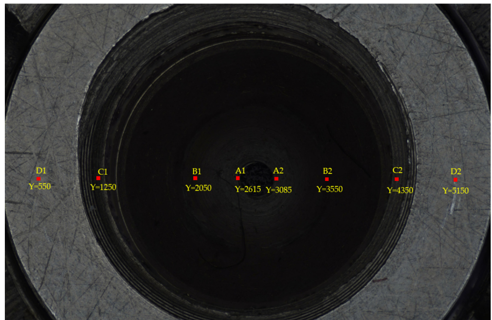
Figure 7. The sharpness evaluation position of the fuel nozzle.
