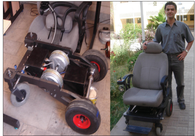
Figure 1: The electric wheelchair constructed in order to experimentally verify the proposed control method
