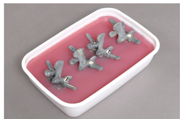
Fig. 2 Third lumbar vertebra sawbone models embedded in Repligel (Swiss-Composite, Fraubrunnen, Switzerland)
