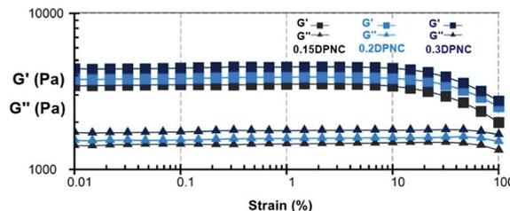
Fig. 12  $G'$  and  $G''$  values of the typical hydrogels (0.15DPNC, 0.2DPNC, and 0.3DPNC), as obtained based on the strain amplitude sweep.
