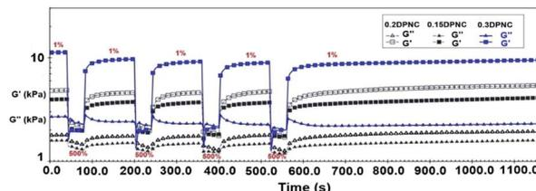
Fig. 13  $G'$  and  $G''$  values estimated based on a continuous strain sweep with the hydrogels alternatively subjected to small (1% strain) and large (500% strain) oscillation forces.
