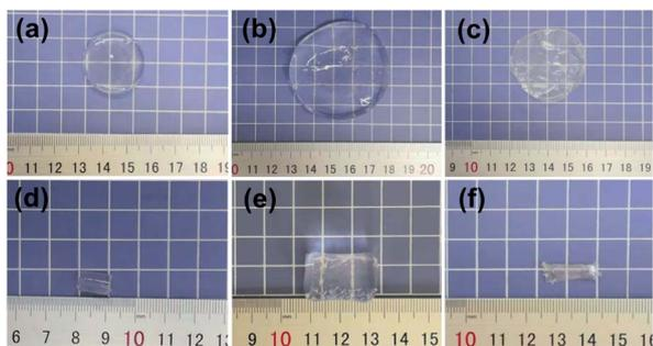
Fig. 3 (a–f) Photo images of the as-prepared 0.2DPNC hydrogel sample (a and d), the swelled 0.2DPNC hydrogel sample after water absorption equilibrium (b and e), and the corresponding oven-dried sample (c and f).
