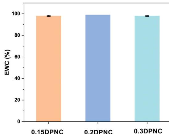
Fig. 5 EWCs estimated for the three representative 0.15DPNC, 0.2DPNC, and 0.3DPNC hydrogel samples.
