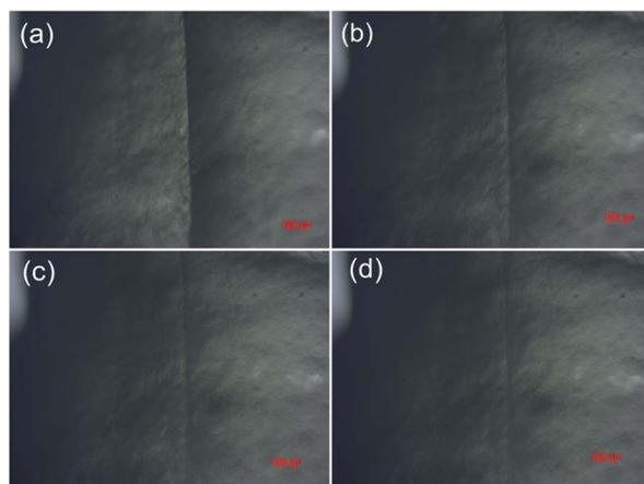
Fig. 10 Metallographic microscope images showing the self-healing process of the typical 0.2DPNC composite hydrogel for different durations: (a) 0 min, (b) 1 min, (c) 2 min, and (d) 3 min test.
