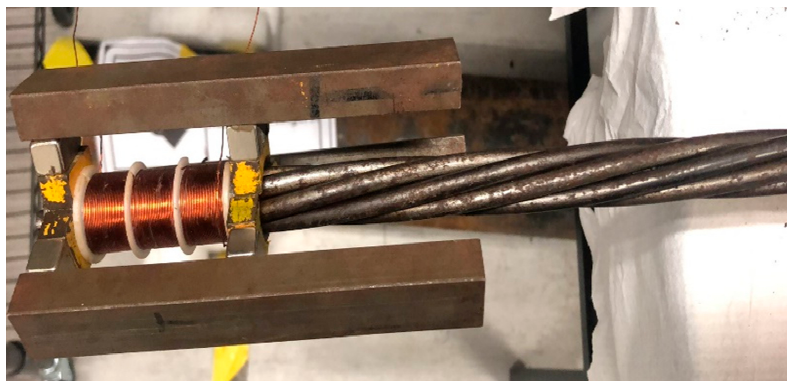
Figure 9. The real configuration of the hard coil Magnetostrictive Sensor (MsS) mounted to the end of the steel strand.
