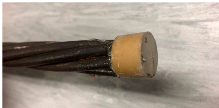
Figure 18. New circular PZT attached to the end of the strand by instant glue.
