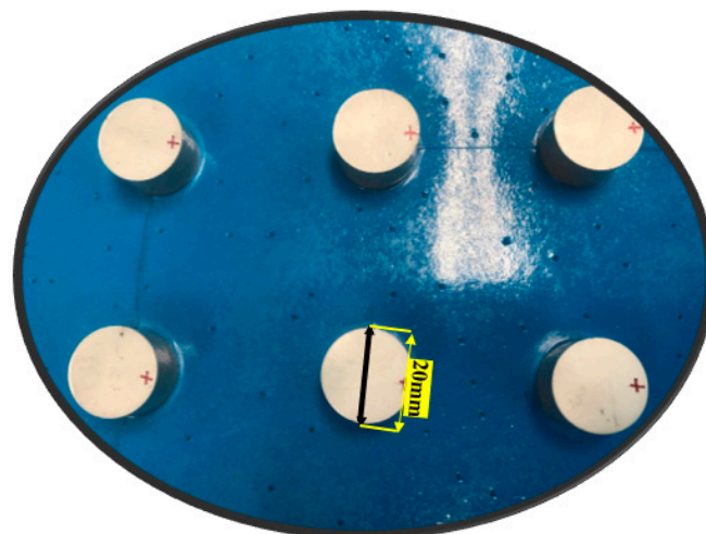
Figure 16. Configuration of PZT used in the experiment.
