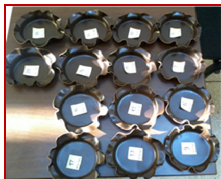
Figure 10. Items moulded from the selected starch-based material with target mineral and renewable fillers, thermoformed at 80 °C.
